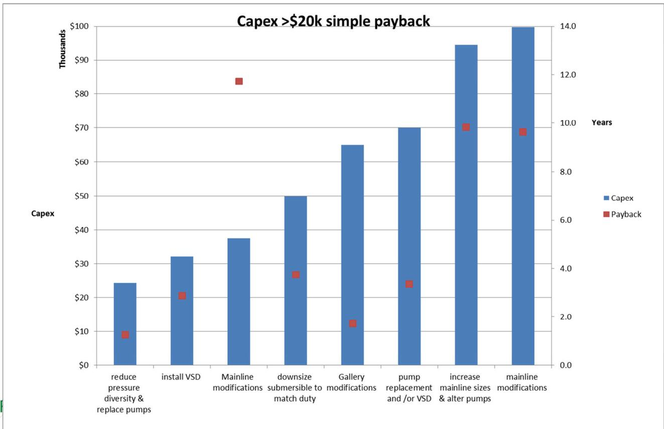
The reports also calculated the costs of pumping a cubic metre (m<sup>3</sup>) of water in kilowatt hours (kWh) and dollars. Where possible this was done to the individual pump. Figure 4 graphs the results.
