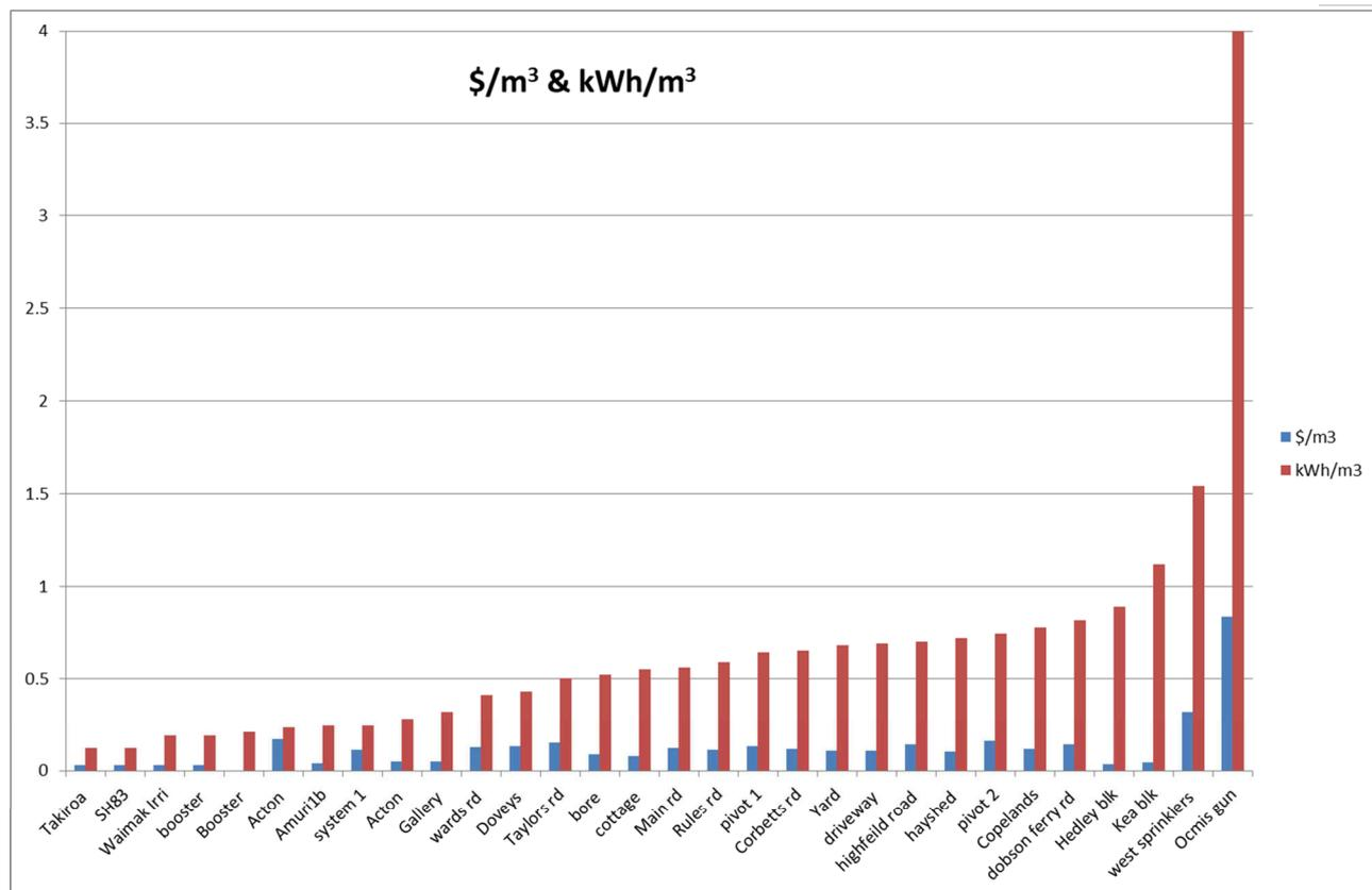
There is a wide range of kWh/m<sup>3</sup> from 0.12 to 4. There will always be a variation as water is pumped from and to, differing heights for each individual irrigation system.
